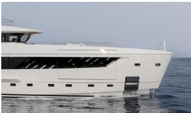
Shell view - With lateral grid Lateral openings = 30%A
